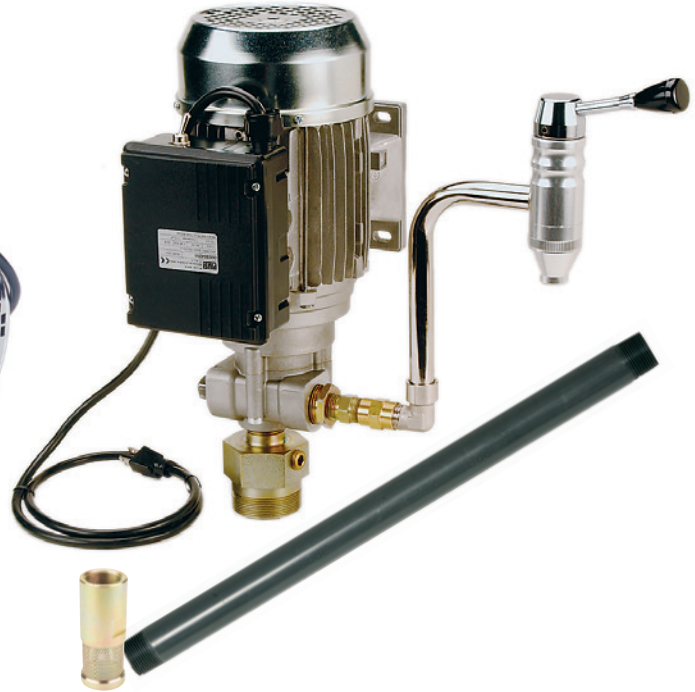
P/N 33221-S3 Vertical mount system includes 3.0 GPM electric pump, spigot, 2" double tap, 1" x 30" suction pipe and foot valve. Ideal for use with 55 gallon drums and bench tanks.
